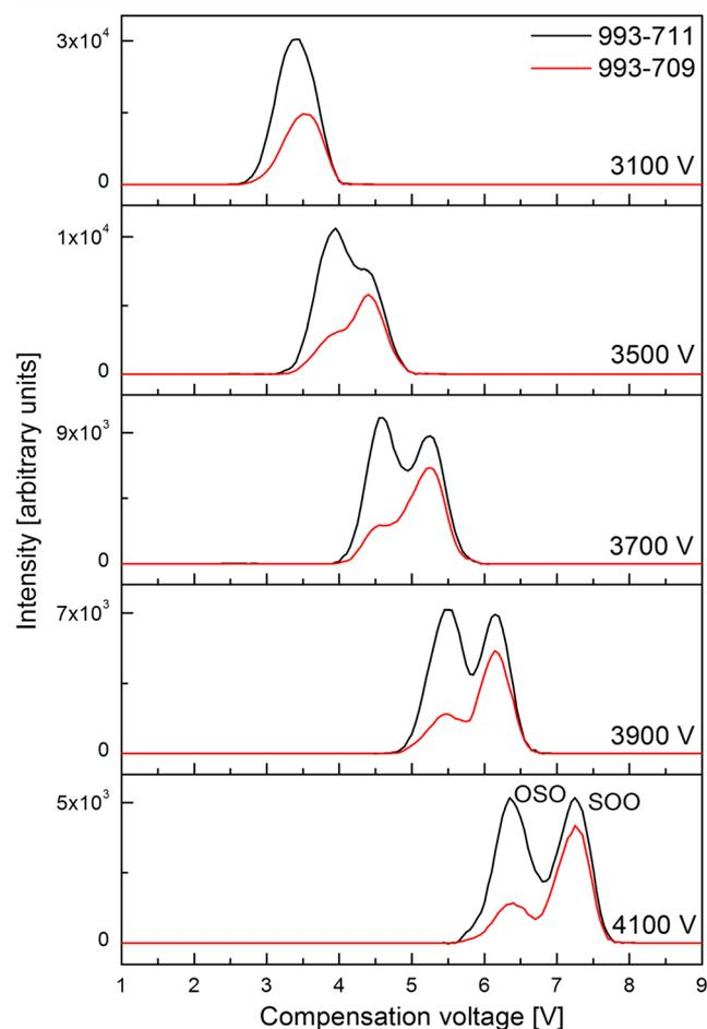
**Figure 3.** Effect of the separation voltage (SV) on the DMS separation of the OSO/SOO regioisomeric pair. The flow rate of 1-propanol as the chemical modifier is 166  $\mu\text{L}/\text{min}$ . Other experimental conditions are the same as for Fig. 1.
