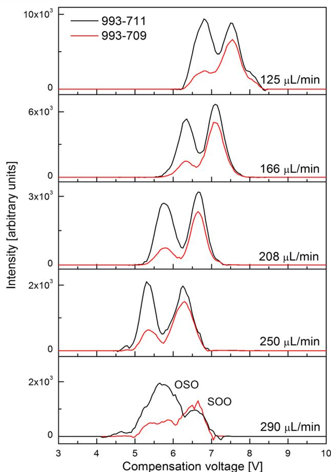
**Figure 2.** Effect of the flow rate of 1-propanol as the modifier in nitrogen as the curtain gas on the DMS separation of the OSO/SOO regioisomeric pair. Other experimental conditions are the same as for Fig. 1.
