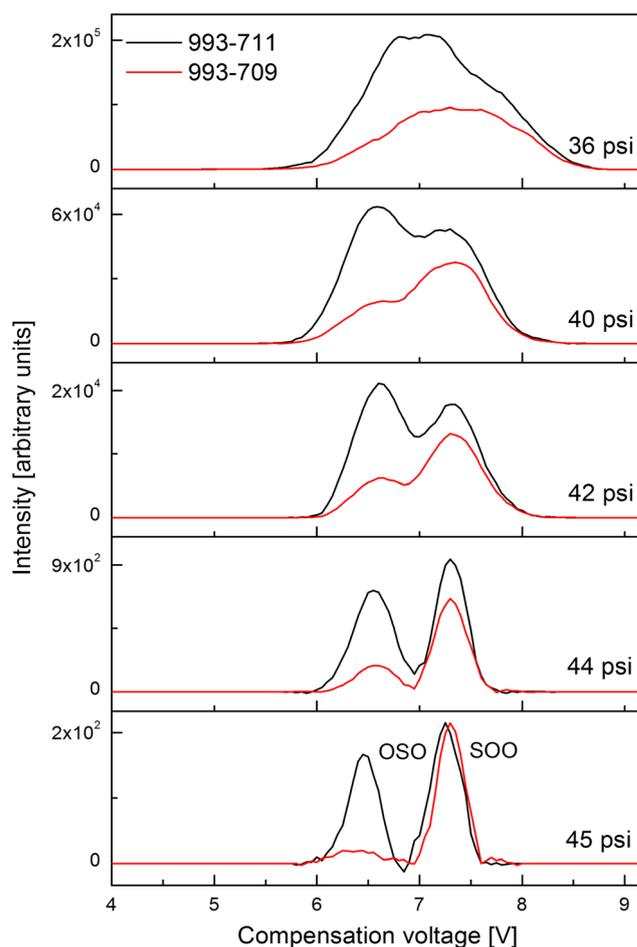
**Figure 4.** Effect of the pressure of throttle gas (DR) on the DMS separation of the OSO/SOO regioisomeric pair using 1-propanol as the chemical modifier and SV 4100 V. Other experimental conditions are the same as for Fig. 3.
