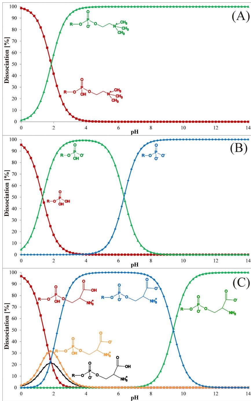
**Fig. 1.** Dissociation equilibria of (A) PC, (B) PA and (C) PS calculated by the Marvin demo software in the pH range 0–14, where R means  $\text{C}_{17}\text{H}_{33}\text{COOCH}_2(\text{C}_{17}\text{H}_{33}\text{COO})\text{CHCH}_2-$ .
