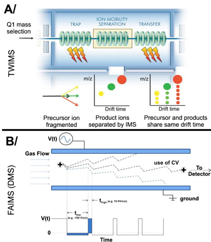
**Fig. 6.** Principles of ion mobility separation of ions in: (A) traveling-wave ion mobility spectrometry (TWIMS) including the scheme of time-aligned parallel (TAP) fragmentation and (B) field-asymmetric waveform ion mobility spectrometry (FAIMS).
