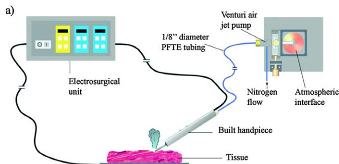
**Fig. 9.** Surgical mass spectrometry: scheme of ion transfer from the tissue to the atmospheric interface to mass spectrometer. Reprinted with a permission from [181].
