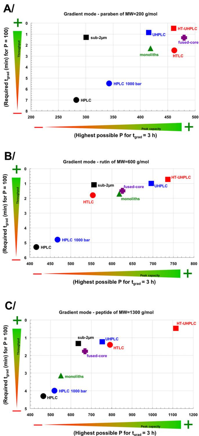
**Fig. 3.** Performance comparison of LC strategies in terms of throughput ( $t_{\text{grad}}$  for  $P=100$ ) and maximum peak capacity ( $P_{\text{max}}$  for  $t_{\text{grad}}=3$  h) in the gradient elution for model compounds: (A) butylparaben (MW=200 Da), (B) rutin (MW=600 Da), and (C) peptide triptorelin (MW=1300 Da).
