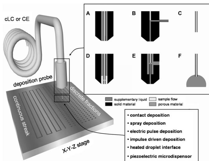
**Fig. 5.** Scheme of off-line LC–MALDI–MS coupling with the supplementary liquid addition and deposition mechanisms. Junctions used for coupling of microcolumn techniques include the following: (A) coaxial sheath flow, (B) T-junction, (C) sheathless interface, (D) porous junction, (E) liquid junction, and (F) droplet electrocoupling. A, B and C are typical for capillary LC–MS, while D, E and F are common in capillary zone electrophoresis–MS.
