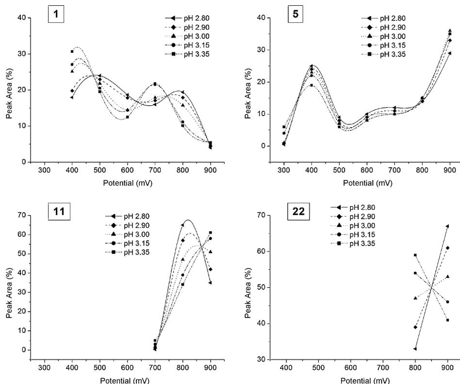
Fig. 2. Effect of the mobile phase acidity on the electrochemical detector response (peak areas) for: 1, gallic acid; 5, gentisic acid; 11, vanillic acid; 22, ethylvanillin.
