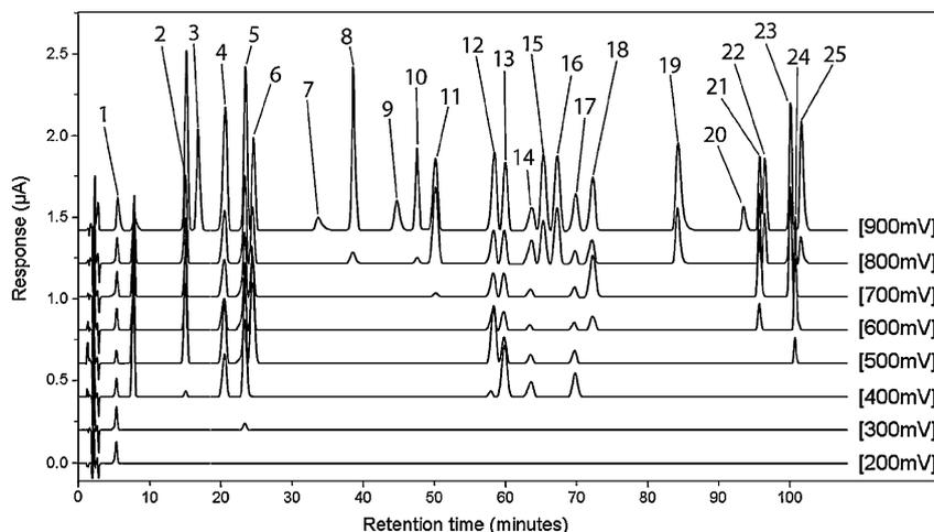
Fig. 3. Chromatographic separation of the phenolic compounds. Experimental conditions: Column Phenomenex Gemini C18 (150 mm  $\times$  3 mm I.D., 3  $\mu$ m particle size), electrochemical detection 200–900 mV (with 100 mV increment), the flow rate 0.45 mL/min, the column temperature 35  $^{\circ}$ C, the injection volume 10  $\mu$ L, the mobile phase gradient 0–27 min, 2% B isocratic; 27–72 min, linear gradient from 2 to 7% B; 72–108 min, linear gradient from 7 to 25% B.
