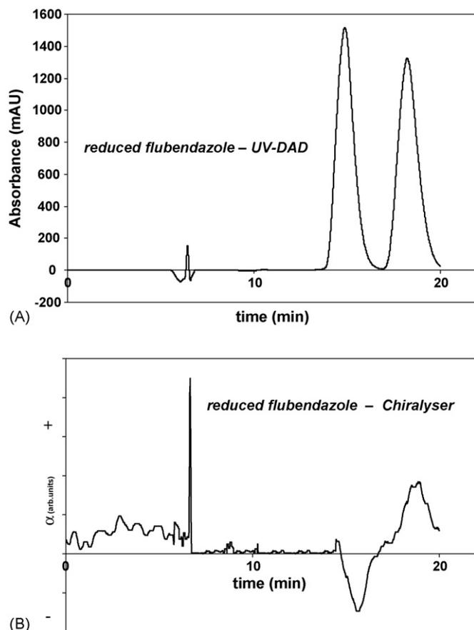
Fig. 5. Chiral analysis of the racemic mixture of (–)-reduced flubendazole ( $t_R = 15$  min) and (+)-reduced flubendazole ( $t_R = 19$  min) by a tandem of UV photodiode-array detector ( $\lambda = 250$  nm, upper graph (A)) and polarimetric Chiralyser detector ( $\lambda = 430$  nm, lower graph (B)).
