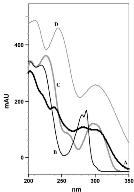
Fig. 3. Characteristic UV spectra of hydrolysed flubendazole (line A,  $\lambda_{\max} = 203, 239, 283, 300$  nm), reduced flubendazole (line B,  $\lambda_{\max} = 202, 220, 280, 287$  nm), albendazole (line C,  $\lambda_{\max} = 204, 227, 296$  nm) and flubendazole (line D,  $\lambda_{\max} = 210, 245, 300$  nm). The spectra were collected during a chromatographic analysis by photodiode array detector (see Section 2.5.1 for the achiral chromatographic conditions).
