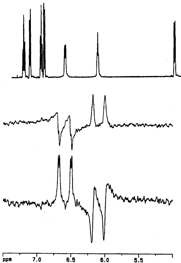
Fig. 4 Part of ^1\text{H} NMR spectrum of compound 7 in \text{DMSO}-\text{D}_6 (top trace) and part 1D gradient selected ^1\text{H}-^{15}\text{N} HMBC spectrum of compound 7 optimized for 90 Hz and measured using ^{15}\text{N} hard pulse (middle and bottom traces). The middle and bottom traces belong to the same 1D ^1\text{H}-^{15}\text{N} HMBC spectrum and traces differ only in phasing performed with aim to correct different off-resonance effects of ^{15}\text{N} hard pulse on appropriate nitrogens
