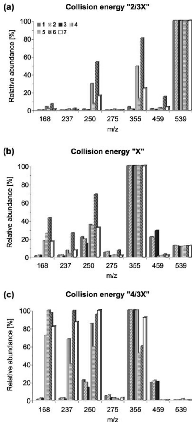
**Figure 3.** Results of inter-laboratory comparison of MS/MS spectra of the  $[M-H]^-$  ion of model compound C.I. Acid Red 118 measured with three collision energies and seven different tandem mass analyzers: (a) collision energy X, (b) collision energy 2/3X, (c) collision energy 4/3X; (1) Esquire 3000 ion trap, (2) Esquire LC ion trap, (3) LCQ ion trap, (4) 1200L triple quadrupole, (5) Micromass Quattro Premier triple quadrupole, (6) QqTOF Ultima API, and (7) QqTOF MicrOTOF-Q.
