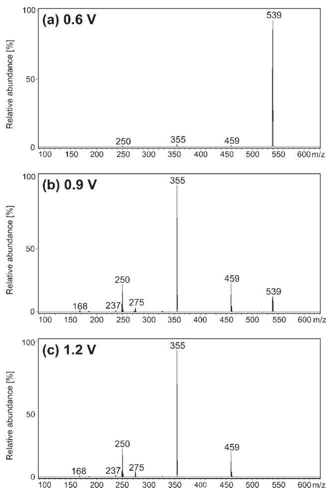
**Figure 2.** Negative ion ESI-MS/MS spectra of the precursor ion  $[M-H]^-$  at  $m/z$  539 using three collision energies measured on the Esquire 3000 ion trap mass spectrometer: (a)  $0.6\text{ V} (=2/3X)$ , (b)  $0.9\text{ V} (=X)$ , (c)  $1.2\text{ V} (=4/3X)$ .
