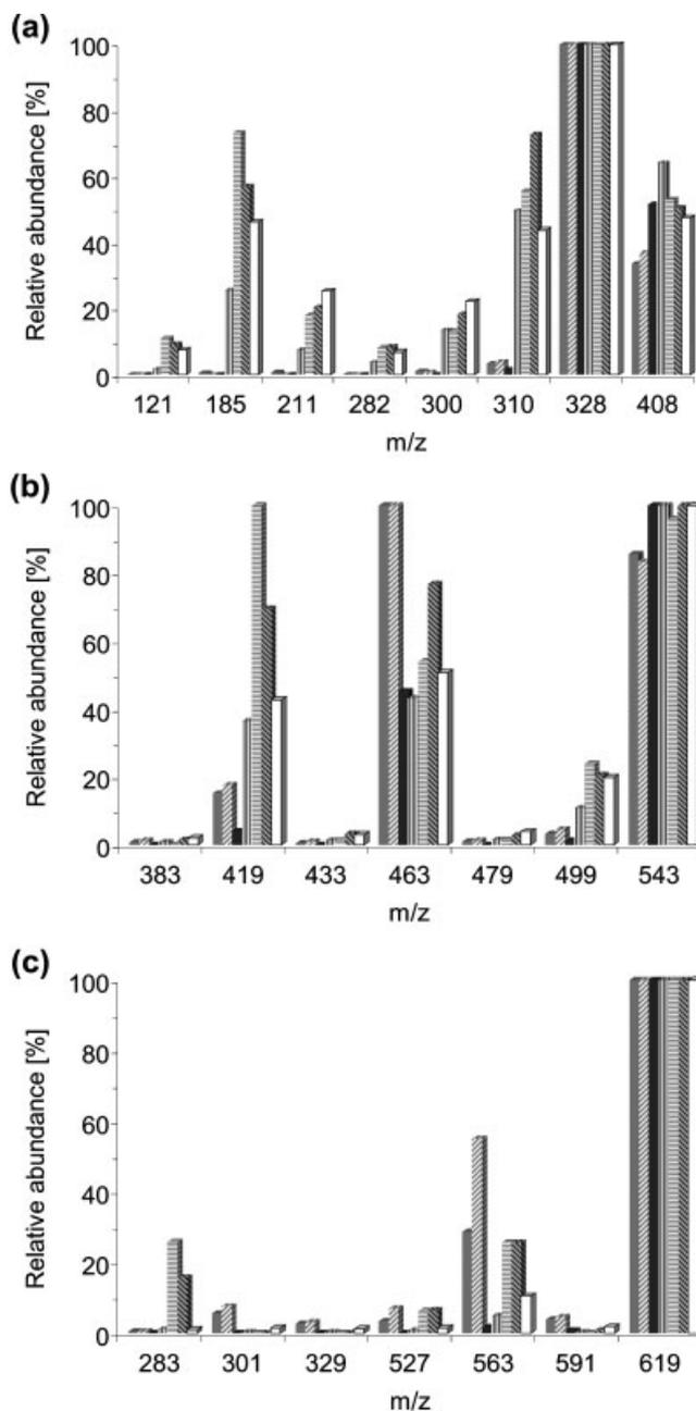
**Figure 5.** Weighted averages ( $X=50\%$ ,  $4/3X=25\%$  and  $2/3X=25\%$ ) of intensities at three collision energies for three representatives of dye classes: (a) C. I. Acid Violet 43 as anthraquinone dye, (b) C. I. Acid Blue 1 as triphenylmethane dye, (c) Al(III) metal-complex azo dye. (1) Esquire 3000 ion trap, (2) Esquire LC ion trap, (3) LCQ ion trap, (4) 1200L triple quadrupole, (5) Micromass Quattro Premier triple quadrupole, (6) QqTOF Ultima API, and (7) QqTOF MicrOTOF-Q.
