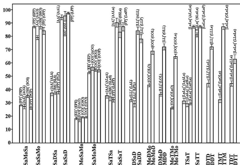
**Fig. 7.** Plots of relative abundances of  $[R_1R_1]^+$  related to  $[R_1R_2]^+$  fragment ions (100%) with their standard deviations for randomization mixtures measured on the single quadrupole mass spectrometer; annotation of x axis: Sa – saturated, Mo – monounsaturated, D – diunsaturated, T – triunsaturated; annotation of particular columns correspond to individual  $[M+H-R_2COOH]^+$  ions fragmented from TGs written in parentheses.
