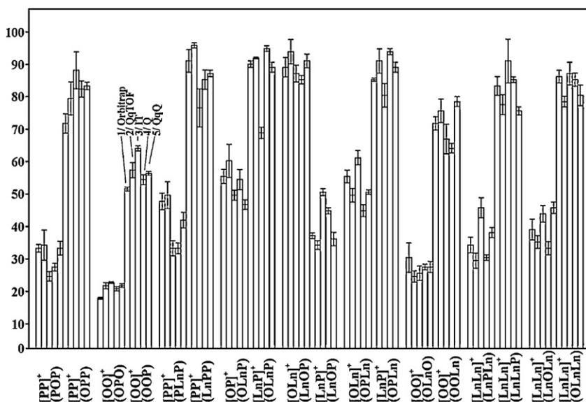
**Fig. 6.** Plots of relative abundances of  $[R_1R_1]^+$  related to  $[R_1R_2]^+$  fragment ions (100%) with their standard deviations for the randomization mixture PPP/OOO/LnLnLn measured on five different instruments: (1) LTQ Orbitrap XL (Thermo Fisher Scientific), (2) quadrupole time-of-flight micrOTOF-Q (Bruker Daltonics), (3) ion trap Esquire 3000 (Bruker Daltonics), (4) single quadrupole LC/MSD (Agilent Technologies) and (5) triple quadrupole API 3000 (AB SCIEX).
