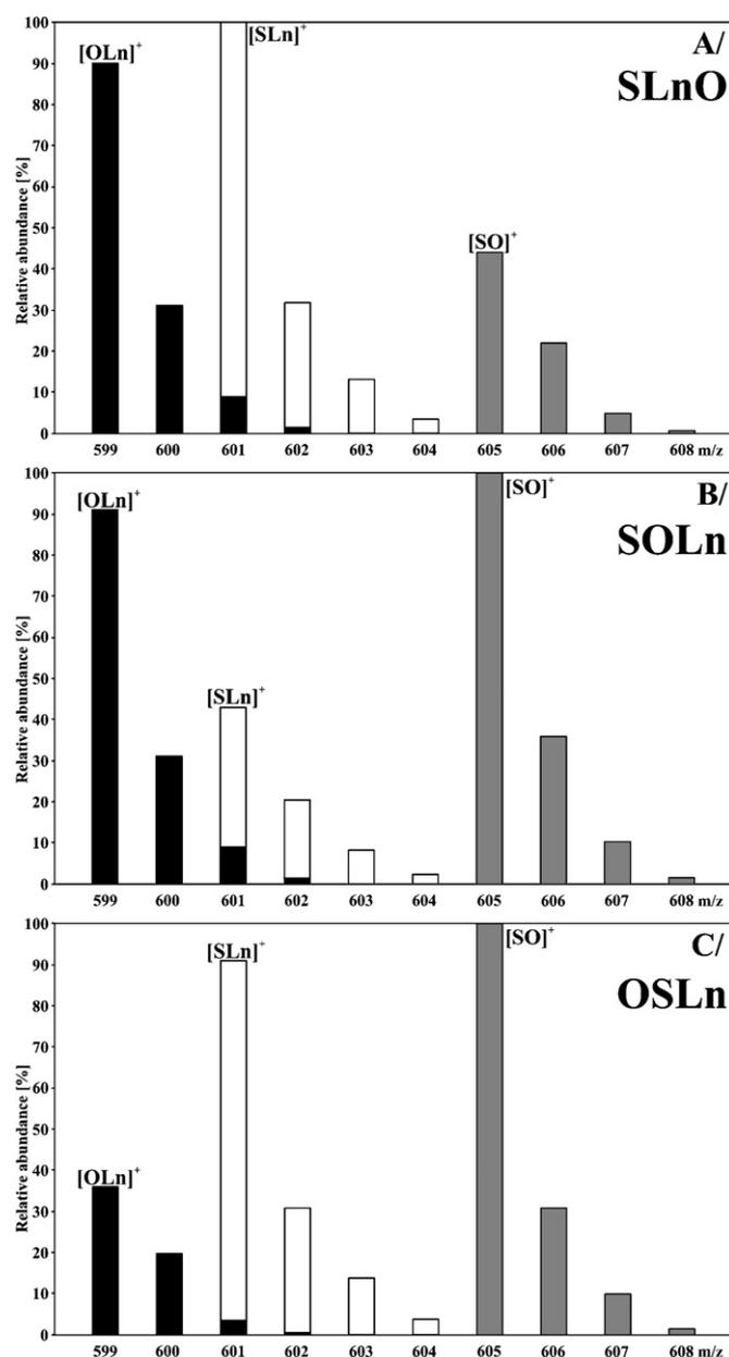
Fig. 2. Normalized relative abundances of  $[M+H-R_1COOH]^+$  fragment ions in APCI mass spectra of regioisomeric triplet SLnO (A), SOLn (B) and OSLn (C) obtained from the chromatogram shown in Fig. 1.
