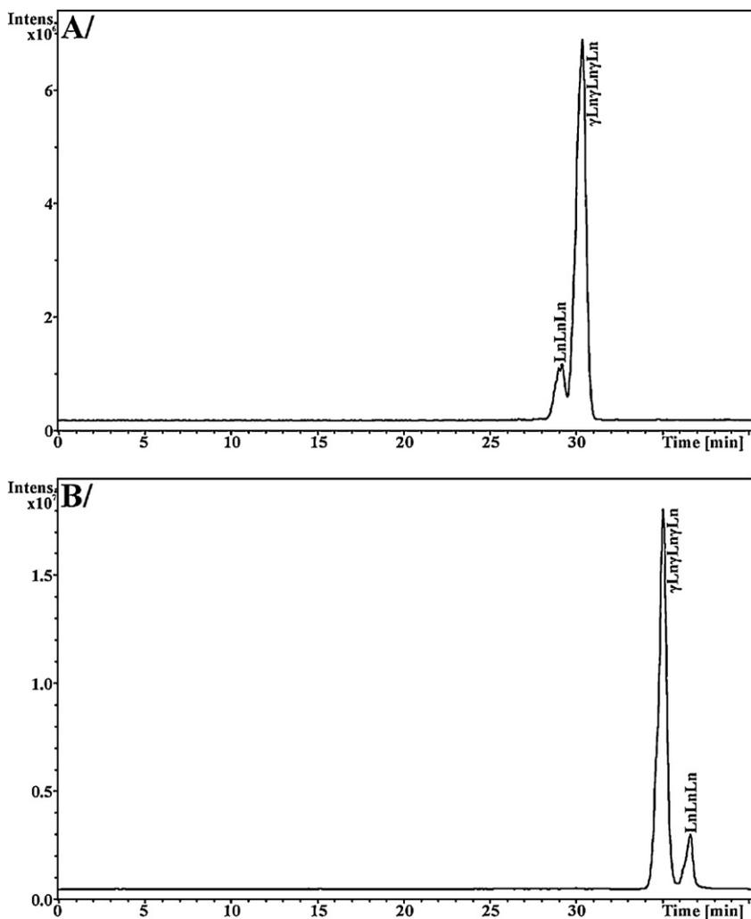
**Fig. 5.** Comparison of retention behavior of LnLnLn and  $\gamma$ LnLnLn in two different mobile phase systems: (A) 0 min – 100% A, 60 min – 50% A + 50% B, where A is hexane–2-propanol–acetonitrile (99.8:0.1:0.1, v/v/v) and B is hexane–2-propanol–acetonitrile (96:2:2, v/v/v) [2] and (B) 0 min – 100% acetone, 5 min – 100% acetone, 30 min – 94% acetone + 7% acetonitrile, 40 min – 89% acetone + 11% acetonitrile [20]. All other experimental conditions are identical as in Section 2.
