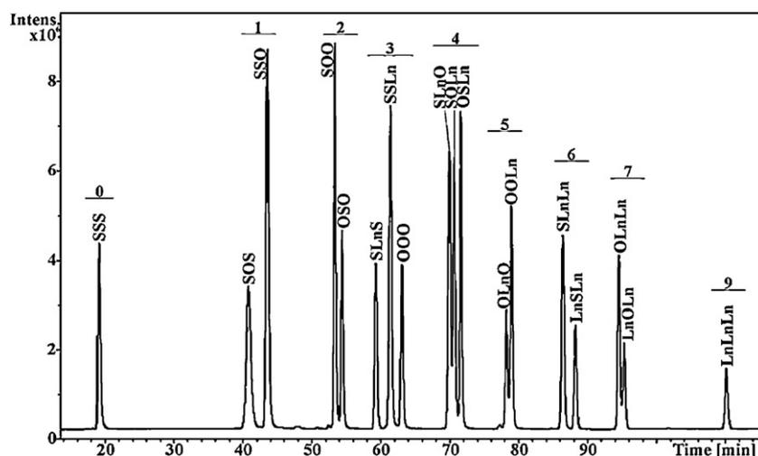
**Fig. 1.** Silver-ion HPLC/APCI-MS chromatogram of the randomization mixture prepared from tristearin (SSS, C18:0), triolein (OOO, Δ9-C18:1) and trilinolenin (LnLnLn, Δ9,12,15-C18:3), see Section 2 for conditions. Numbers correspond to the double bond number.
