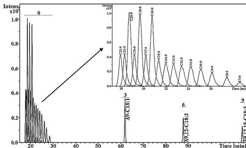
**Fig. 4.** Silver-ion HPLC/APCI-MS chromatogram of all mono-acid TG standards. Numbers correspond to the double bond number. Inset zoom shows the resolution of saturated TGs from C7:0 to C22:0. Concentrations of all standards are identical except for C16:0, C18:0 and C20:0 with doubled concentrations.
