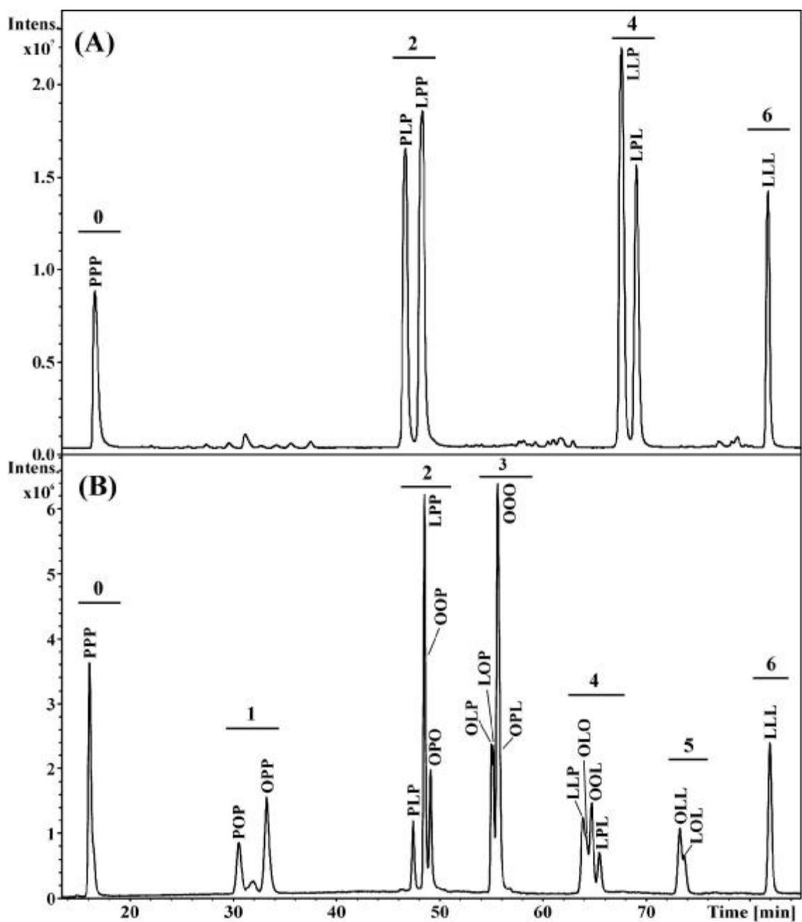
**Figure S2.** Silver-ion HPLC/APCI-MS analysis of randomization mixtures: (A) PPP / LLL, (B) PPP / OOO / LLL. Chromatographic conditions are described in the Experimental section.
