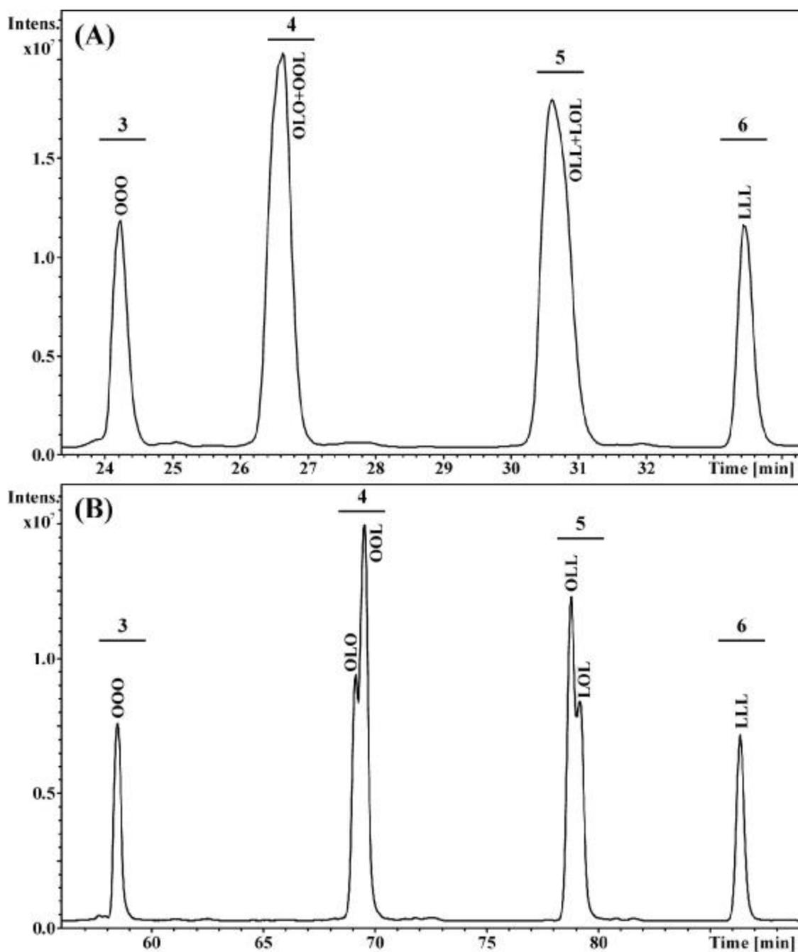
**Figure S1.** Effect of the column length on silver-ion HPLC/APCI-MS analysis of TGs in the randomization mixture of OOO/LLL: (A) one 25 cm ChromSpher Lipids column, (B) three 25 cm ChromSpher Lipids columns connected in series. Chromatographic conditions are described in the Experimental section.
