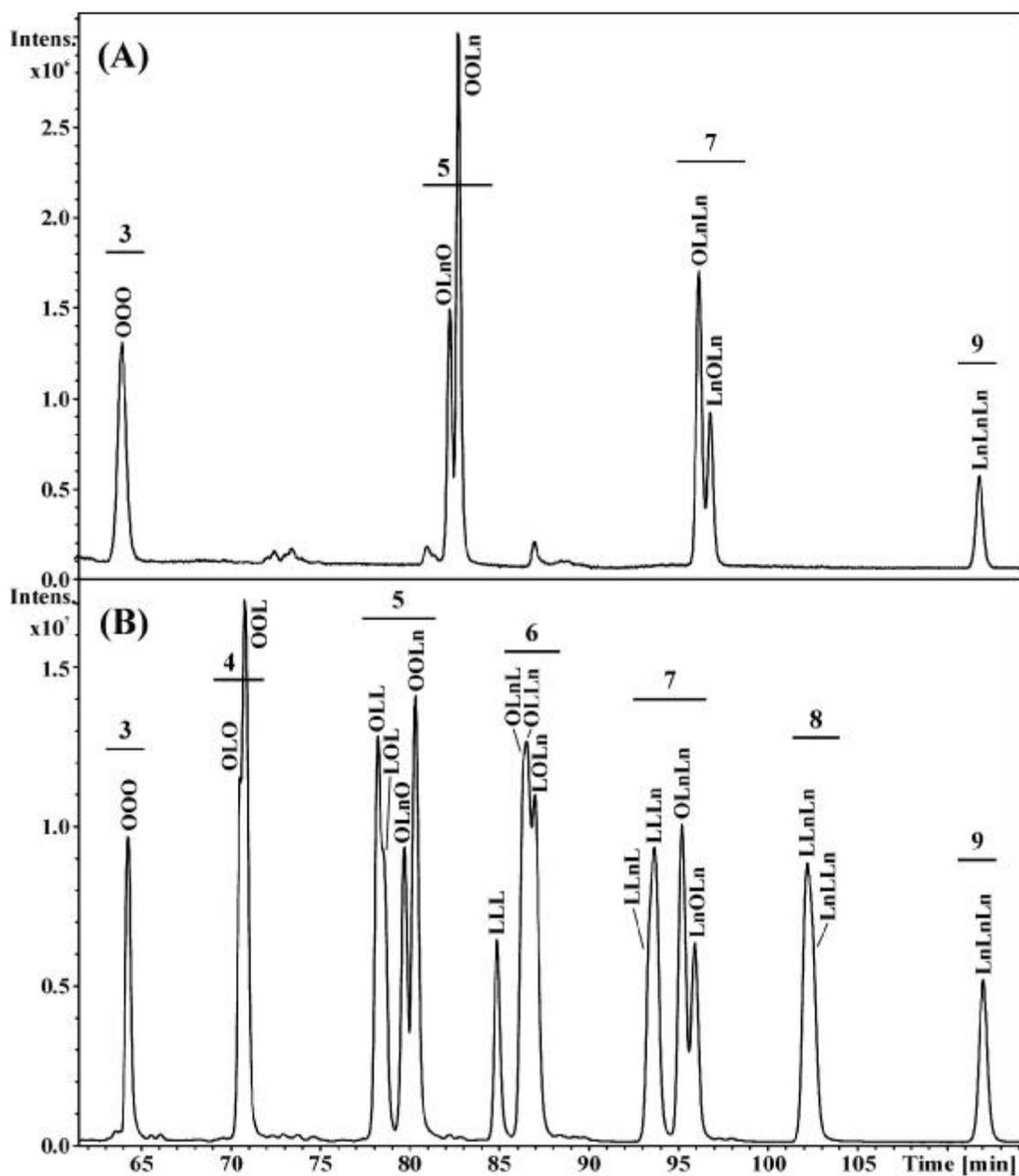
**Figure S3.** Silver-ion HPLC/APCI-MS analysis of randomization mixtures: (A) OOO / LnLnLn, (B) OOO / LLL / LnLnLn. Chromatographic conditions are described in the Experimental section.
