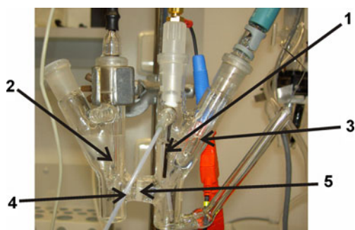
Fig. 2 Schematic diagram of electrochemical H-type cell: 1, working electrode (glassy carbon or pyrolytic graphite electrode); 2, auxiliary electrode (platinum sheet); 3, reference electrode (Ag/AgCl/3 mol L -1 KCl); 4, inlet of argon for bubbling; 5, glass frit
